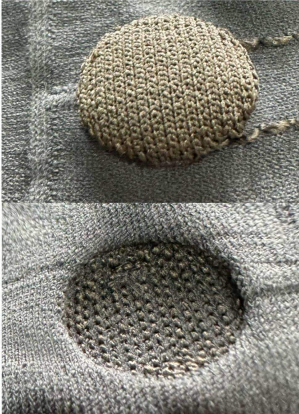
Figure 3-4. 3D knitted silver electrode. (Top) Back side of the knitted fabric. (Bottom) Front side of the knitted fabric.
