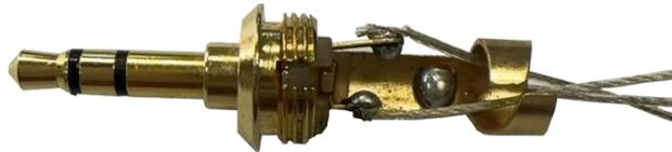
Figure3-13 3.5 mm jack plug with conductive wires
