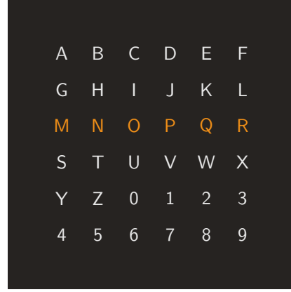
(b) The P3 matrix speller interface. Entire rows or columns flash at once.
