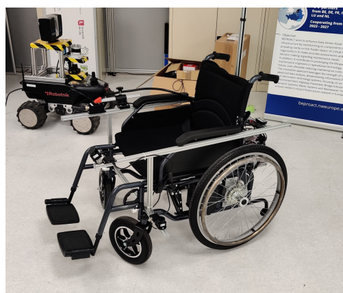
(d) Motorized wheelchair for controlled physical movement
