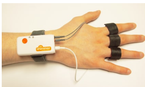
(c) Shimmer3 GSR sensor for physiological monitoring 3
