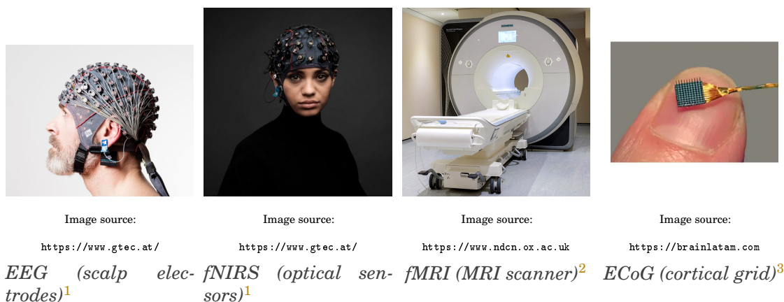
Figure 1.2: Illustrative hardware for common brain measurement modalities: EEG uses scalp electrodes; fNIRS uses near-infrared optical sensors; fMRI uses a high-field magnetic resonance scanner; ECoG uses electrode grids on the cortical surface (invasive).
