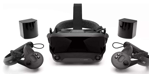
(b) Valve Index VR headset with tracking cameras and controllers 2
