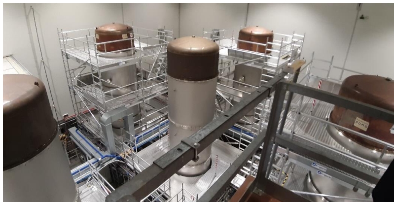
Fig. 8 Towers containing the superattenuators and the mirrors. The 5 towers are under vacuum and each contain a superattenuator from which the mirrors are suspended and controlled by the marionetta. The towers from left to right contain the: Power Recycling Mirror, (West) Input Mirror, Beam Splitter, (North) Input Mirror, Signal Recycling Mirror. Source: Photo taken by Philippe Vincent
