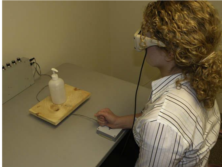
Figure 19. The experimental setup used by Jax & Buxbaum (2010). The participant wears occlusive eye glasses. Participant's right-hand rests on a button device during experimental sessions. Objects are positioned in front of the participants. At the signal (i.e., when eye glasses open), participants are asked to position their hand on the object as if they were going to grasp or use it, depending on the condition. Time between the signal and the onset of the movement (i.e., initiation time) are recorded. Figure from Jax & Buxbaum (2010).
