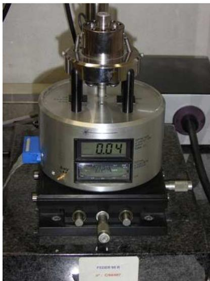
FIG. 1.14 – Microscope AFM Multimode.
