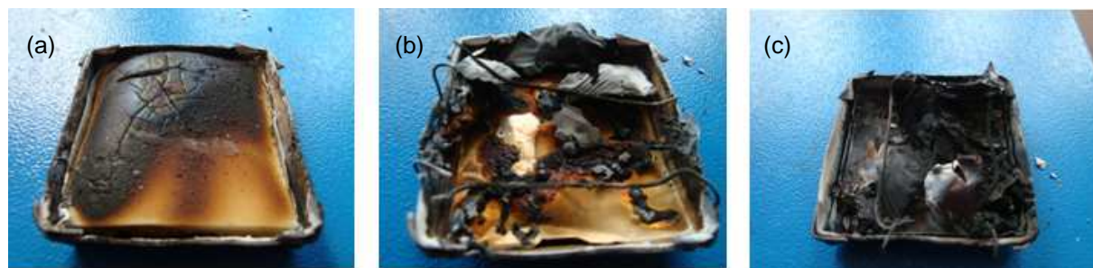
Fig. 150: Mass loss calorimeter residues of vulcanized EVM/OP1230 collected before ignition (a), at PRHR (b) and at the end of combustion(c)
