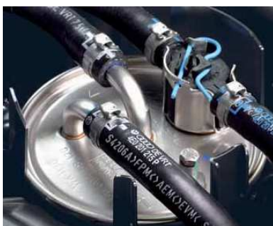
Fig. 21: Fuel hoses made of EVM (Levapren®)
