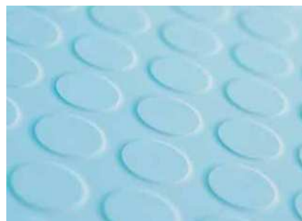
Fig. 22: Floor covering made of EVA (Levapren®)
