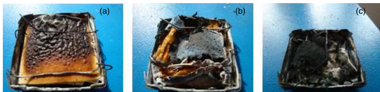
Fig. 151: Mass loss calorimeter residues of vulcanized EVM/ATH/OP1230 collected before ignition (a), at PRHR (b) and at the end of combustion(c)
