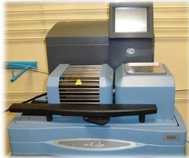
**Figure 42.** ATG couplée DSC Q600 (TA Instruments)
