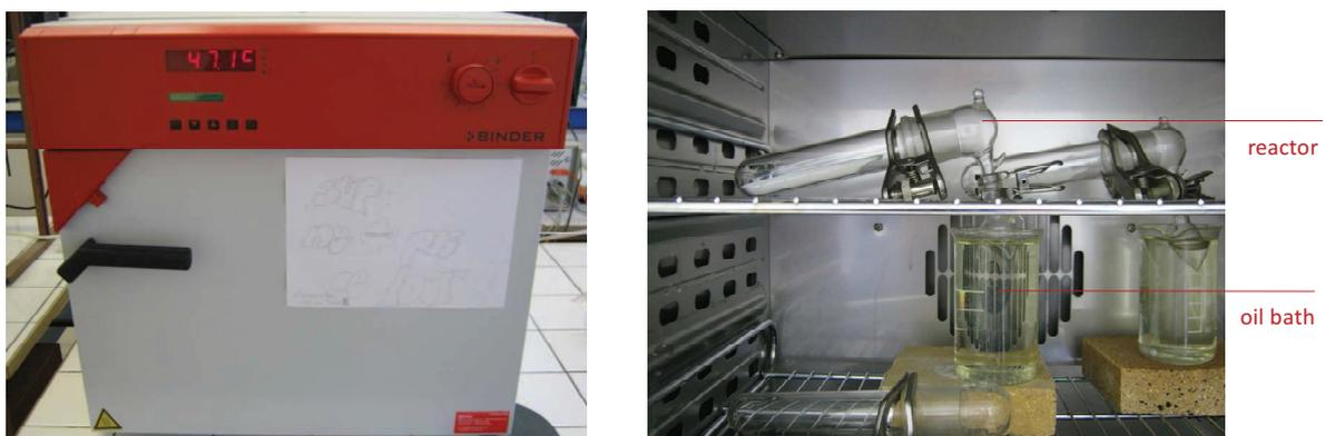
Fig. 2.17: Left side: Incubator oven used for weathering assays. Right side: View inside the incubator oven. Reactor systems were placed on two grill levels. Ventilation (see rear wall) was used to homogenize the temperature inside the oven. The water reservoirs were kept in oil baths during weathering.
