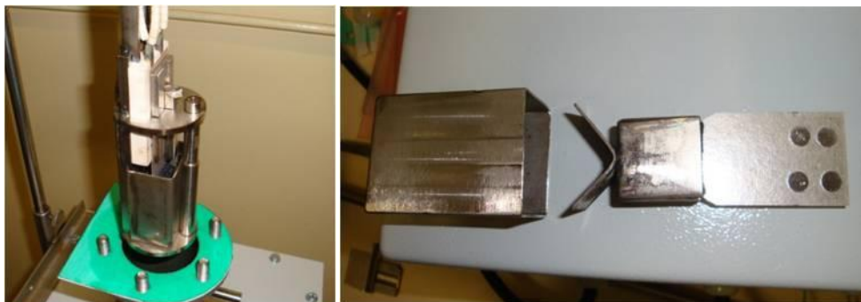
Figure 53: Furnace (left) and sample holder (right) of TPS2500
