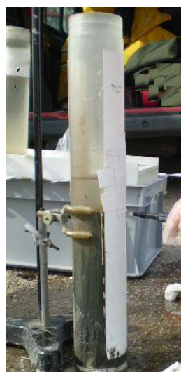
Figure III. 3: Collection of sediment cores and measurement of redox potential.
