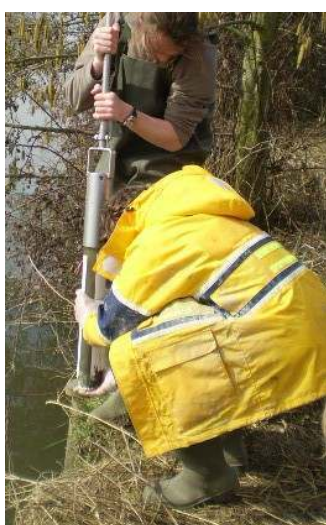
Figure III. 3: Collection of sediment cores and measurement of redox potential.
