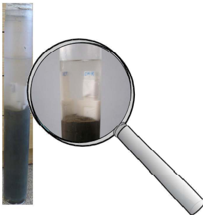
Figure V. 8: Deployment of DGT probes into the sediment
