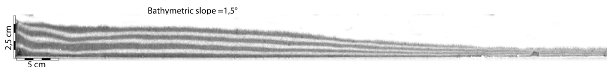
Figure 3. Regional cross section of an undeformed experimental fan built by 7 consecutive flows. Note the very gentle bathymetric slope (Vertical exaggeration X2).
