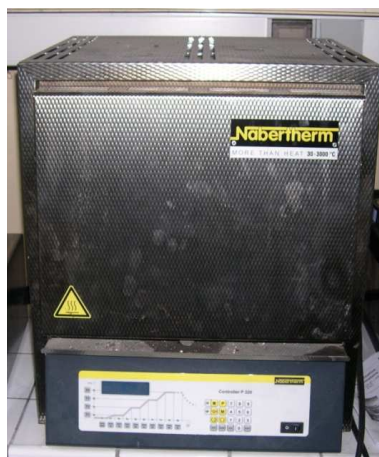
Figure VIII.7 : Four de recuit Nabertherm LT24/11
