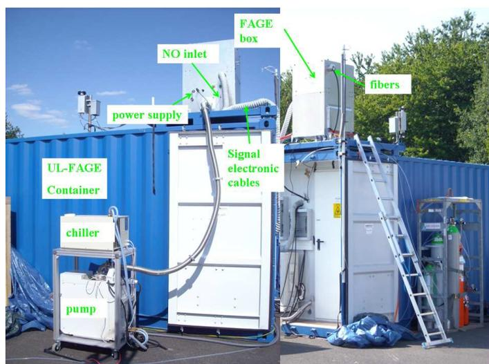
Figure 10. UL-FAGE container during CompOH. The FAGE box is placed on top of the container.
