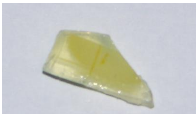
Figure III. 1 Yellow color observed in the irradiated area (60 mW of pulsed femtosecond laser)
