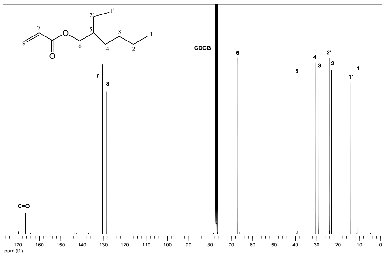
Figure 5.8: ^{13}\text{C} NMR spectra of poly 2-ethylhexyl acrylate PEHA polymer.
