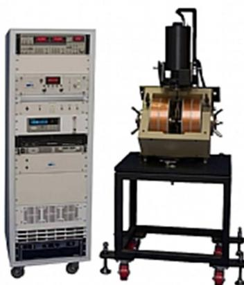
*Figure 13: Vibrating sample magnetometer*
