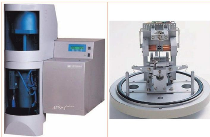
Figure 4: Thermogravimetric analyzer
