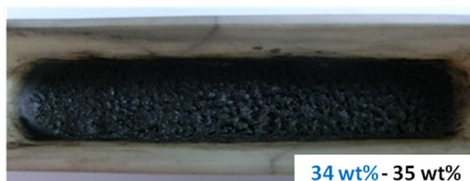
Figure 78 : Picture of the residue of PBT/GF obtained after thermal treatment to 600°C in nitrogen. In blue: expected mass loss (according to TGA), in black: experimental mass loss
