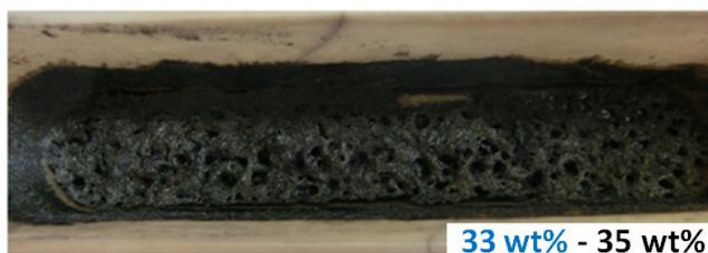
Figure 93 : Picture of the residue of PBT/GF/ C9 obtained after thermal treatment to 600°C in nitrogen. In blue: expected mass loss (according to TGA), in black: experimental mass loss
