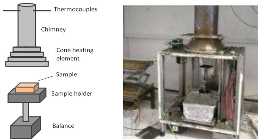
Figure 44 : Schematic representation of a mass loss calorimeter
