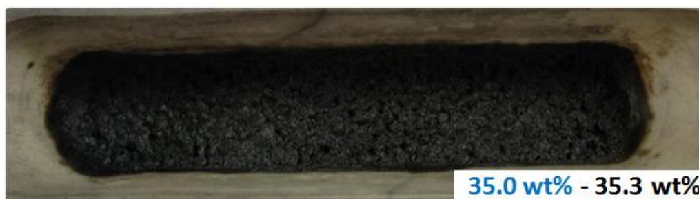
Figure 108 : Picture of the residue of PBT/GF/OP1240 obtained after thermal treatment at 600°C in nitrogen. In blue: expected mass loss (according to TGA), in black: experimental mass loss
