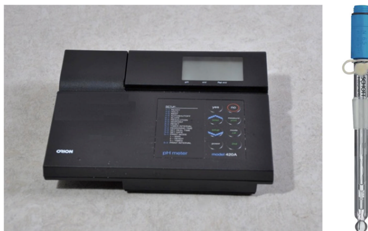
Figure 0.3 Picture of the Orion 420A (left) and of the Schott Silamid® N65 electrode (right)
