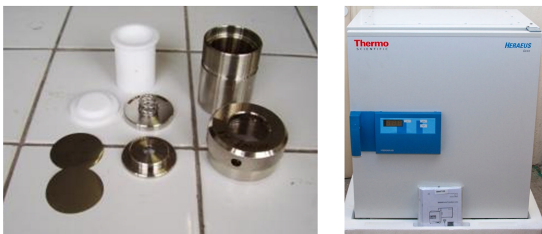
Figure 0.1 Pictures of Parr type autoclave (left) and Heraeus® oven (right) employed in the hydrothermal syntheses of the uranyl coordination polymers.
