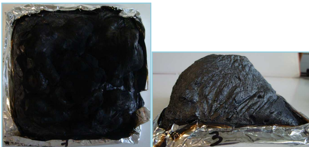
Figure 142: Picture of the PU 28%APP 2%nano SiO 2 residues at the end of a cone calorimeter test
