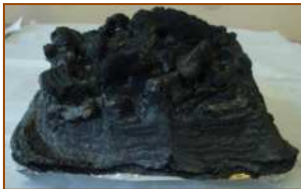
Figure 146: Picture of the PU 28%APP 2% nano gold residue at the end of a cone calorimeter test
