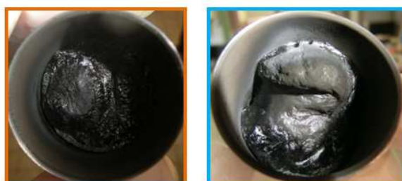
Figure 156: Pictures of residues collected after degradation with method MLCi-Q-AT-o (left: PU 30%APP, right: PU 28%APP 2%nano MgO)
