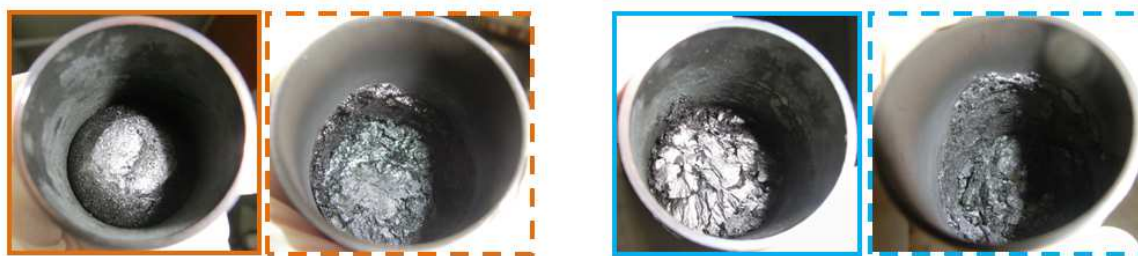
Figure 158: Pictures of residues collected after measuring the strength as a function of gap on samples prepared by methods RF-HR500-500-o (full line) and MLCi-Q-AT-o (dash line) (left: PU 30%APP, right: PU 28%APP 2% nano MgO)
