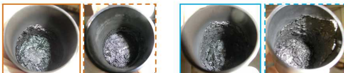
Figure 154: Pictures of residues collected after measuring the strength as a function of gap on samples prepared by methods MLCi-Q-AT-o (full line) and MLCøi-Q-AT-o (dash line) (left: PU 30%APP, right: PU 28%APP 2%nano MgO)
