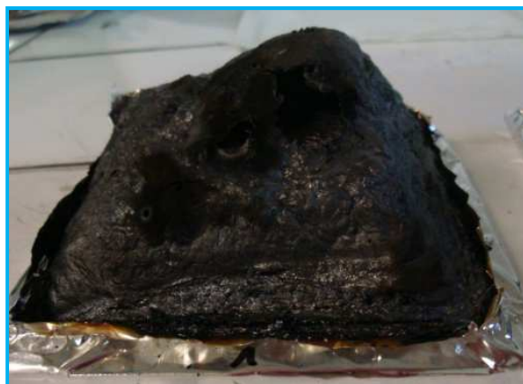
Figure 139: Picture of the PU 28% APP 2% nano MgO residue at the end of a cone calorimeter test
