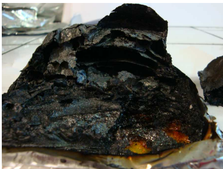
Figure 66: Picture of a slice of PU 28%APP 2% nano MgO residue taken at the end of cone calorimeter showing on the top the char and at the bottom some residual polymer
