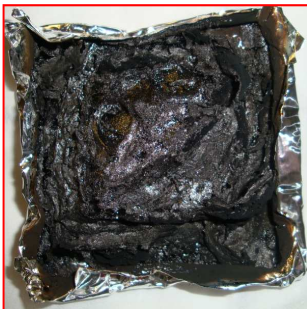
Figure 135: Picture of the PU residue at the end of a cone calorimeter test
