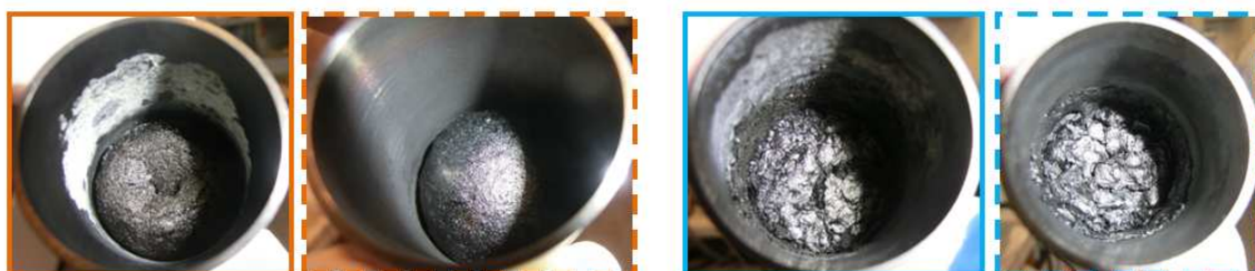
Figure 166: Pictures of residues collected after measuring the strength as a function of gap on samples prepared by methods TO-HR700-AT-o (full line) and TO-HR500-AT-o (dash line) (left: PU 30%APP, right: PU 28%APP 2%nano MgO)
