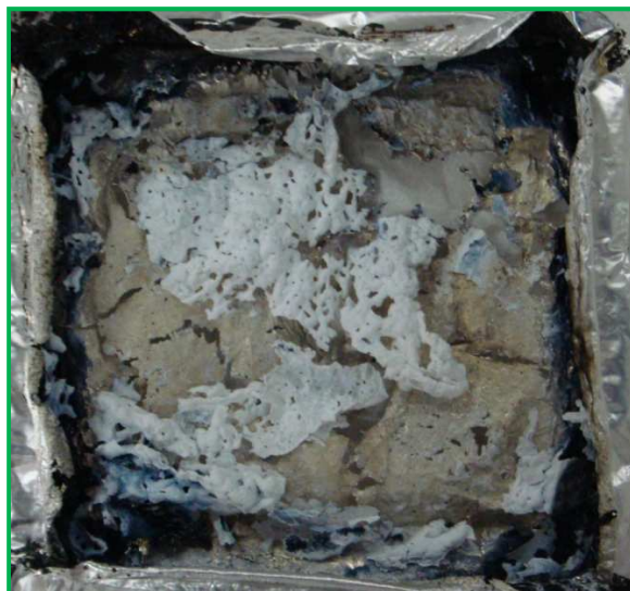
Figure 137: Picture of the PU 5% nano MgO residue at the end of a cone calorimeter test
