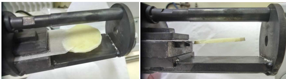
Figure 43: PU sample polymerized on the mica sensor and place on the sample holder to measure the thermal conductivity as a function of temperature
