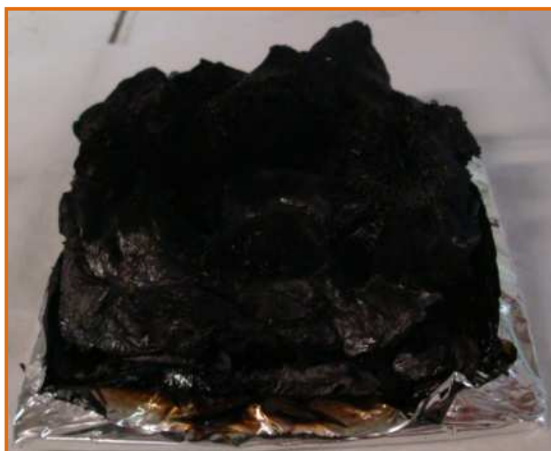
Figure 136: Picture of the PU 30%APP residue at the end of a cone calorimeter test
