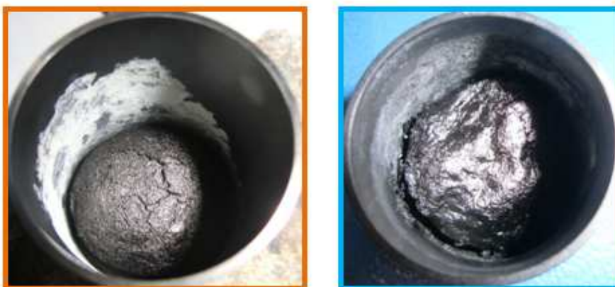
Figure 174: Pictures of residues collected after degradation with method TO-HR700-AT-o (left: PU 30%APP, right: PU 28%APP 2% nano MgO)
