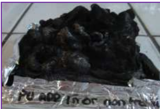
Figure 145: Picture of the PU 29%APP 1% nano gold residue at the end of a cone calorimeter test
