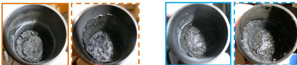
Figure 168: Pictures of residues collected after measuring the strength as a function of gap on samples prepared by methods TO-Q700-AT-o (full line) and TO-Q500-AT-o (dash line) (left: PU 30%APP, right: PU 28%APP 2%nano MgO)
