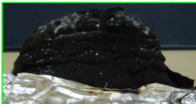
Figure 140: Picture of the PU 25%APP 5%nano MgO residue at the end of a cone calorimeter test
