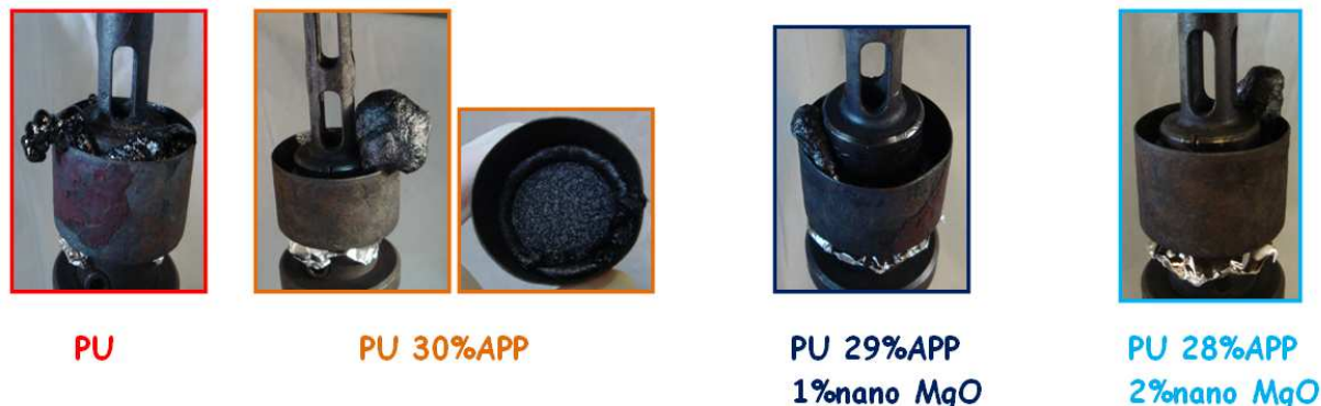
Figure 113: Pictures of the residues at 500°C from PU formulations collected after rheological measurements in a high temperature rheometer
