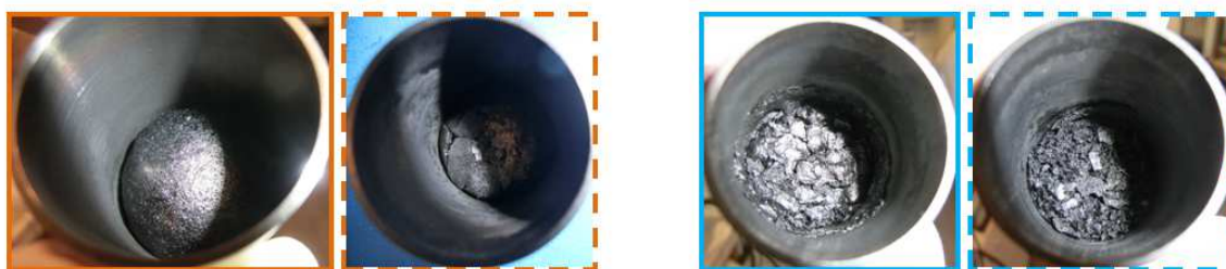
Figure 162: Pictures of residues collected after measuring the strength as a function of gap on samples prepared by methods TO-HR500-AT-o (full line) and RF-HR500-AT-o (dash line) (left: PU 30%APP, right: PU 28%APP 2%nano MgO)
