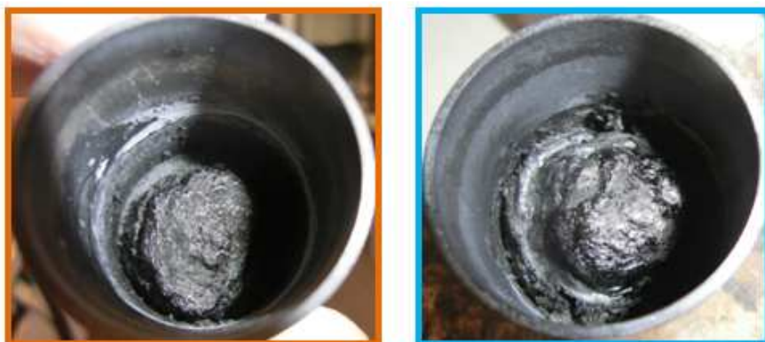
Figure 176: Pictures of residues collected after degradation with method TO-Q700-AT-o (left: PU 30%APP, right: PU 28%APP 2% nano MgO)
