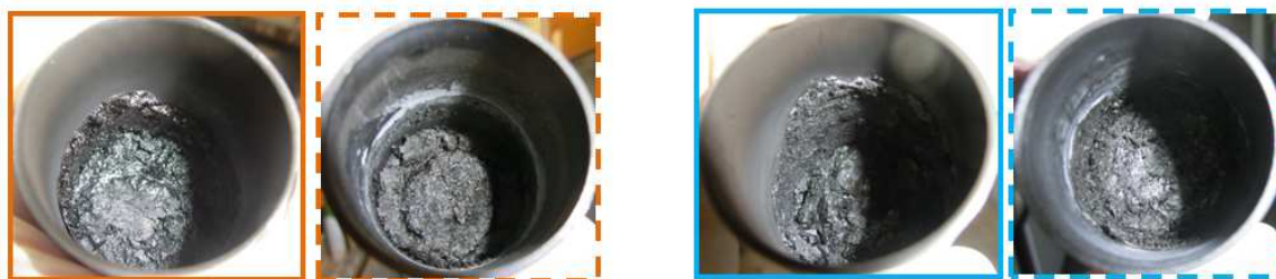
Figure 160: Pictures of residues collected after measuring the strength as a function of gap on samples prepared by methods MLCi-Q-AT-o (full line) and TO-Q700-AT-o (dash line) (left: PU 30%APP, right: PU 28%APP 2% nano MgO)
