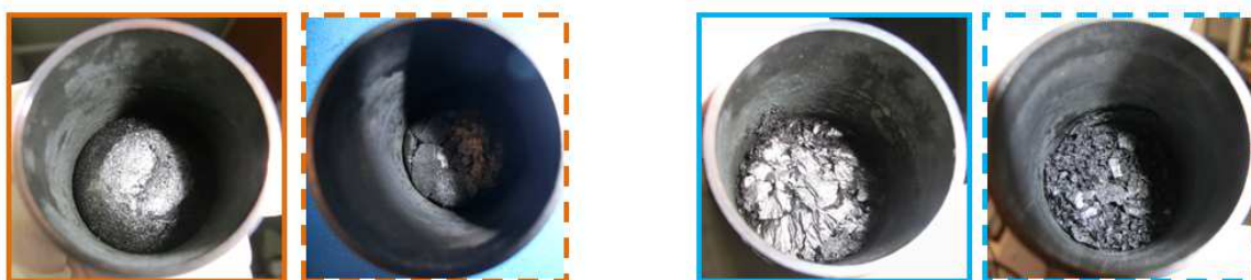
Figure 164: Pictures of residues collected after measuring the strength as a function of gap on samples prepared by methods RF-HR500-500-o (full line) and RF-HR500-AT-o (dash line) (left: PU 30%APP, right: PU 28%APP 2%nano MgO)
