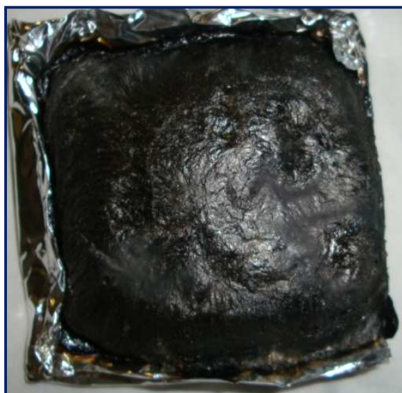
Figure 138: Picture of the PU 29% APP 1% nano MgO residue at the end of a cone calorimeter test
