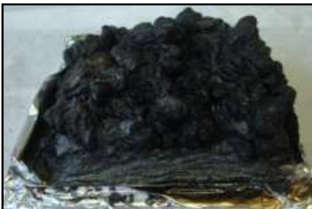
Figure 144: Picture of the PU 29.5%APP 0.5% nano gold residue at the end of a cone calorimeter test
