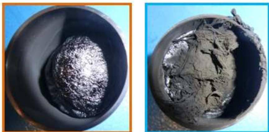
Figure 177: Pictures of residues collected after degradation with method TO-Q500-AT-o (left: PU 30%APP, right: PU 28%APP 2% nano MgO)
