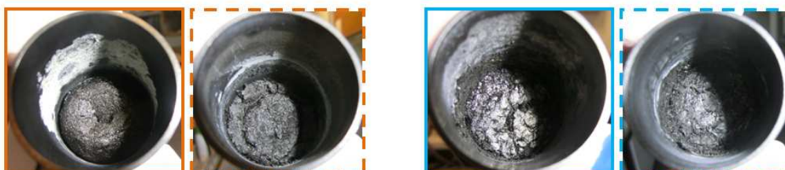
Figure 170: Pictures of residues collected after measuring the strength as a function of gap on samples prepared by methods TO-HR700-AT-o (full line) and TO-Q700-AT-o (dash line) (left: PU 30%APP, right: PU 28%APP 2% nano MgO)
