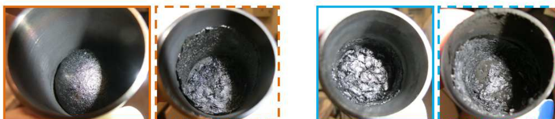
Figure 172: Pictures of residues collected after measuring the strength as a function of gap on samples prepared by methods TO-HR500-AT-o (full line) and TO-Q500-AT-o (dash line) (left: PU 30%APP, right: PU 28%APP 2%nano MgO)
