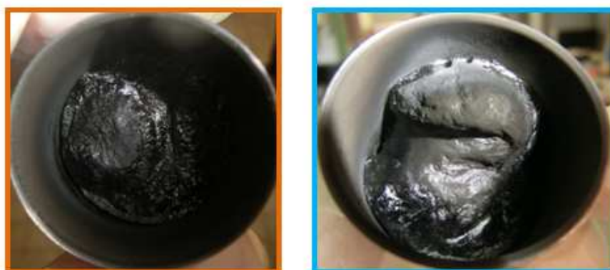
Figure 173: Pictures of residues collected after degradation with method MLCi-Q-AT-o (left: PU 30%APP, right: PU 28%APP 2% nano MgO)
