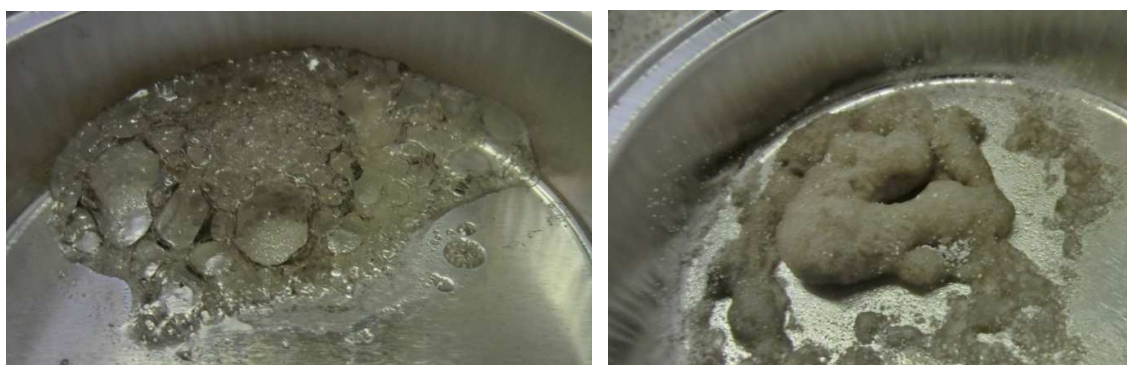
Figure 126: Residue picture after a thermal treatment from 25 to 400°C at 10°C/min on APP (right) and 28%APP 2% nano MgO (left)
