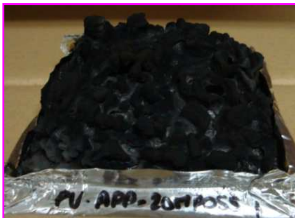
Figure 143: Picture of the PU 28%APP 2%OMPOSS residue at the end of a cone calorimeter test
