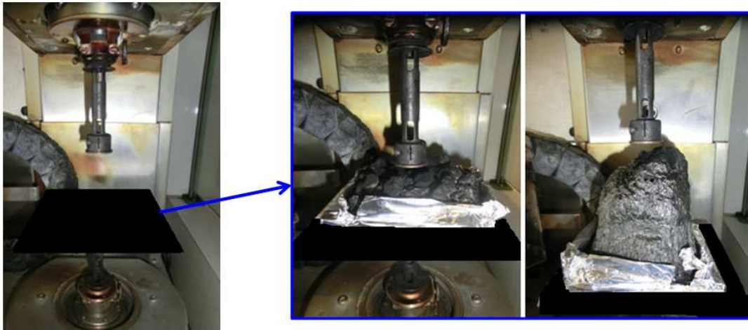
Figure 48: Picture of the device set up to place the mass loss cone calorimeter char on the rheometer in a parallel plate configuration
