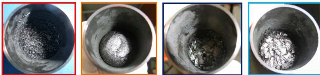
Figure 130: Pictures of residues collected after measuring the strength as a function of gap on samples prepared by the method RF-HR500-500-o (from left to right: PU, PU 30%APP, PU 29%APP 1% nano MgO, PU 28%APP 2% nano MgO)
