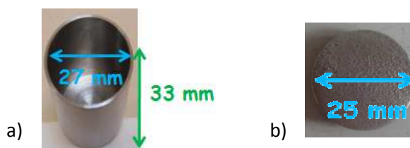
Figure 46: Sample holders used for the bottom (a) and the top (b) plates during rheological measurement
