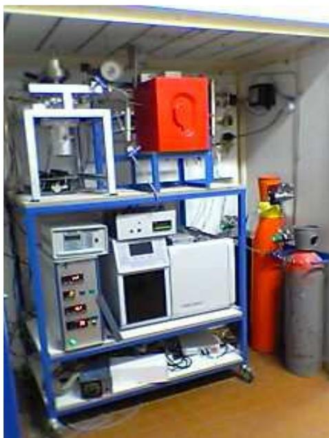
**Figure 2.8** Overview of slurry reactor pilot used for FT synthesis.
