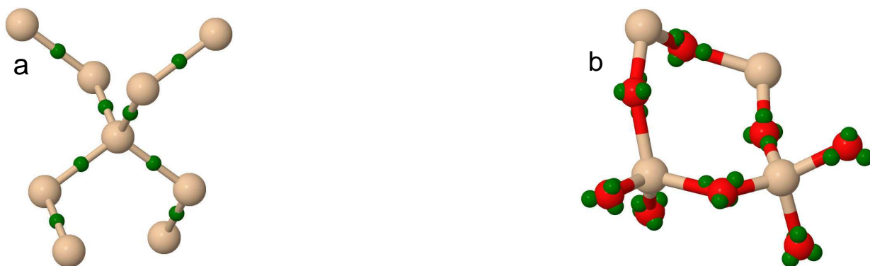
Figure 5.1: Position of Wannier function centers in crystalline silicon (a) and in amorphous silica (b) (fragments of structures are shown). The silicon and oxygen atoms, and Wannier function centers are the wheat, red, and small green balls, respectively.
