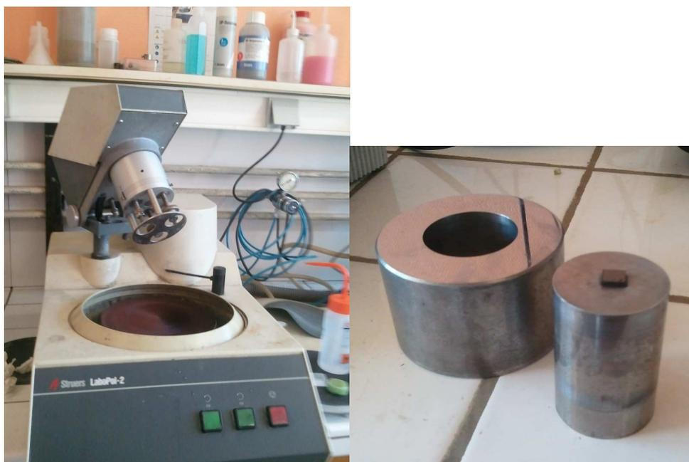
Figure 3.17: (a) Polisseuse semi-automatique Struers LaboPol-2. (b) Piston support de polissage.
