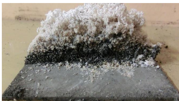
Figure 66: Residue of F4 based coating after hydrocarbon fire exposure
