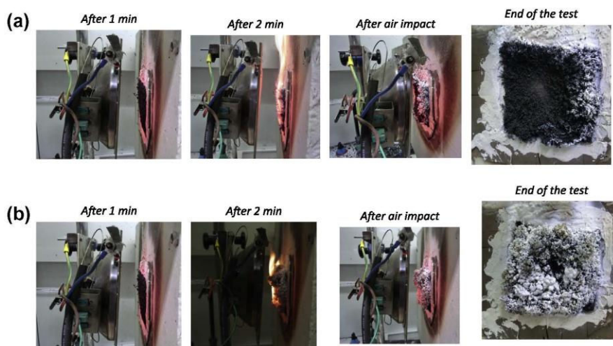
Fig. 7. Fire behavior of (a) S1-Sn/EG and (b) S1-Ti/EG based coating in air jet.
