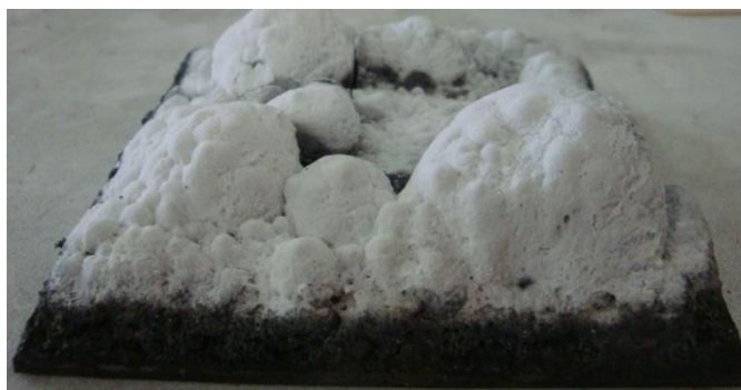
Figure 5 : Typical char obtained at high temperature (expansion about 2800%)
