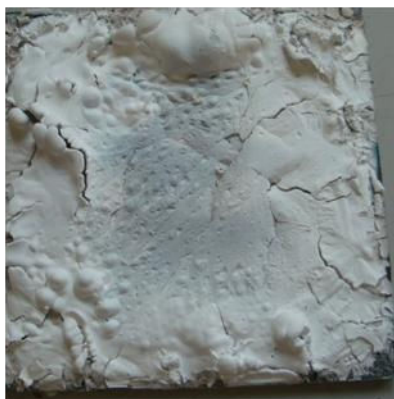
Figure 31: S2/GCC residue after furnace test in cellulosic fire scenario
