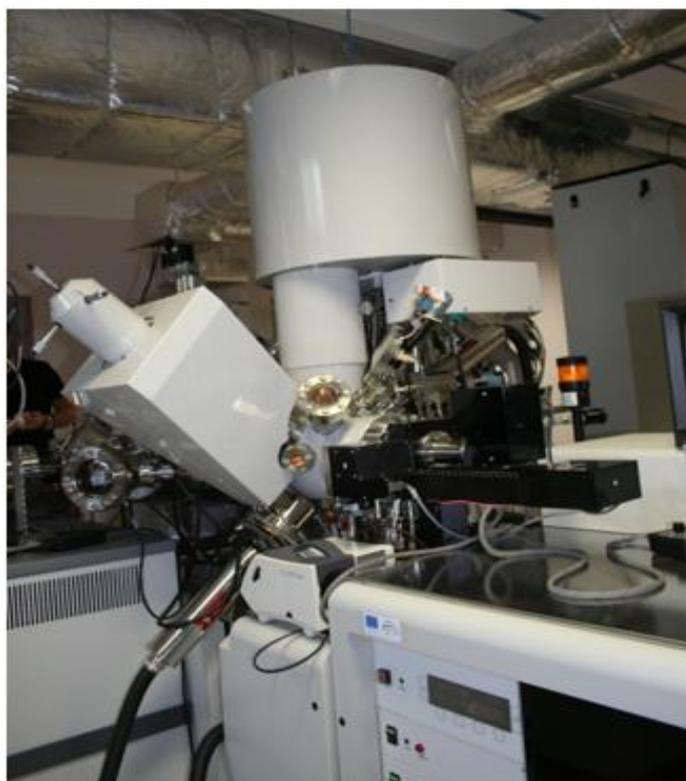
Figure 2-4 X-ray photoelectron spectrometer used for our studies.
