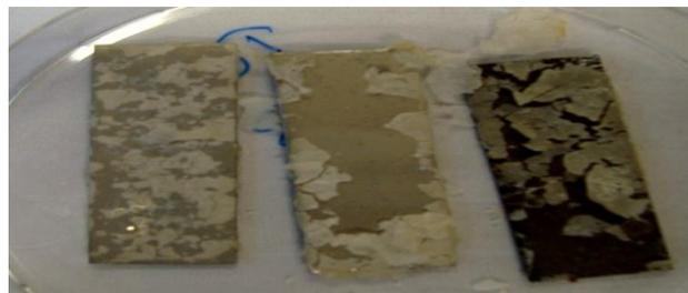
Figure 4.12: The HMDSO coating substrates after Laboratory fouling test.
