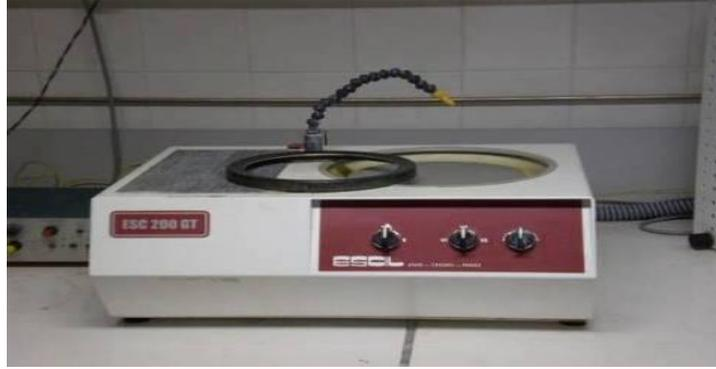
Figure 2.15: Mechanical polishing instrument.
