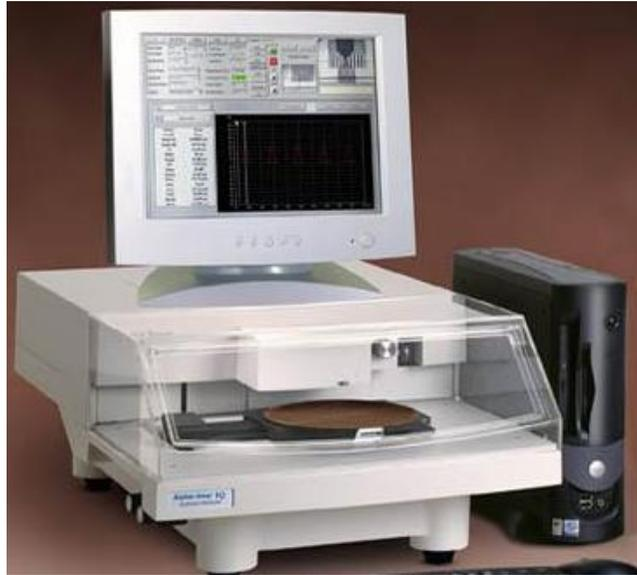
Figure 2.11: Profilometer (Tencor Alpha- Step IQ, Science).
