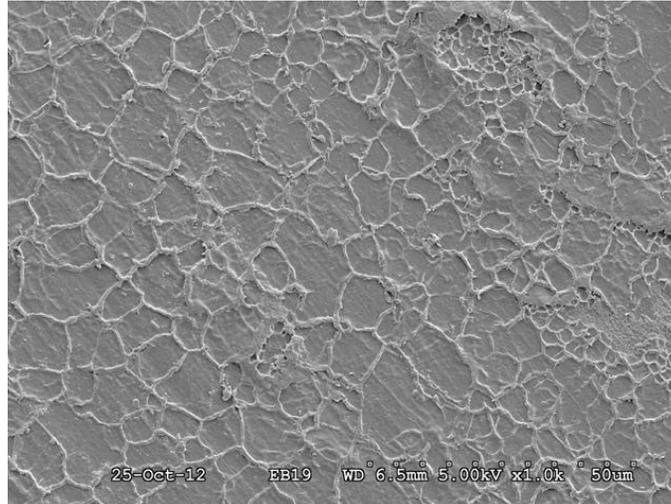
Figure 3.12: SEM analysis of the steel surface when the main fouling layer has been removed
