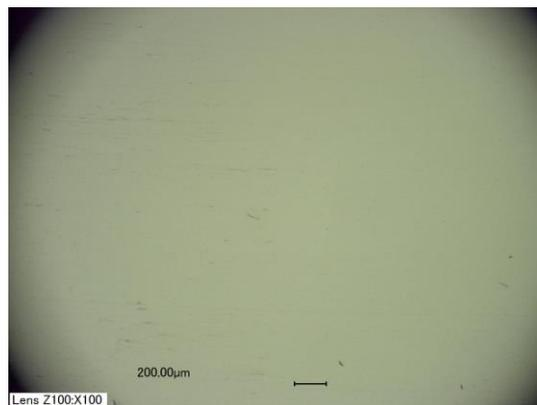
Figure 3.34: The optical microscopic photograph of mirror like stainless steel.
