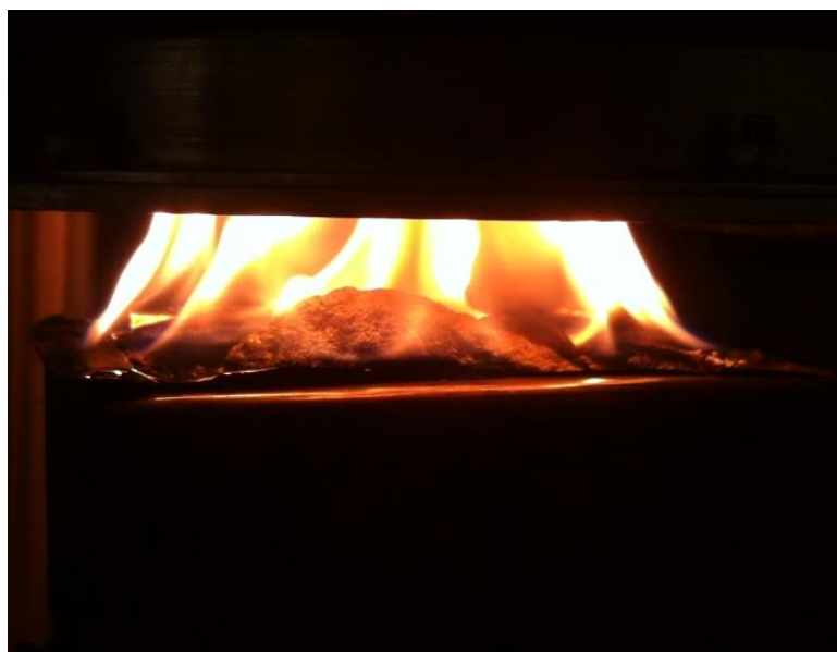
Figure 88: Char formation during the cone calorimetry experiment on PA6/GAS 2.5%/MPP 2.5%
