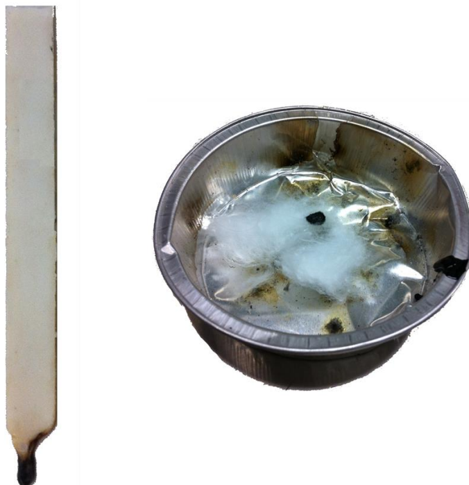
Figure 91: PA6/GAS 2.5%/MPP 2.5% UL94 sample and cotton after test
