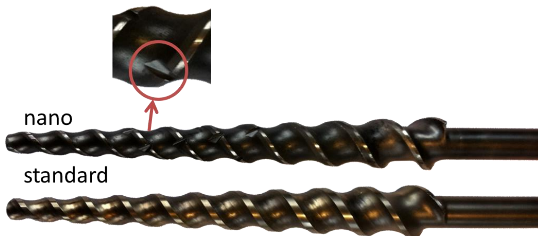
Figure 43: Standard and "nano" screws used with the microextruder, the red circle on the zoomed part shows the notch on the "nano" screws
