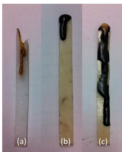
Figure 90: PA6 sample tested at OI below 28 vol.-% (a) PA6/GAS 2.5%/MPP 2.5% sample tested at OI between 23-30 vol.-% (b) and between 31-36 vol.-% (c)
