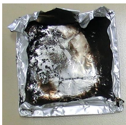
Figure 87: Cone calorimetry residues of PA6 viewed from above
