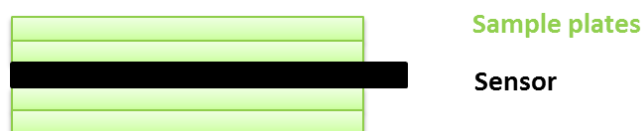
Figure 34: Arrangement of sample plates and sensor for thermal conductivity measurement
