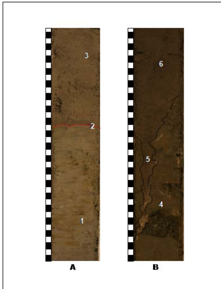
Figure 3.6. Core images from Bierre 3 (A) and Bierre 4 (B) showing the characteristics of the Pleistocene deposits in the subsurface of the FFCP. Scale in centimetres. A Greyish clayey silt with rust-coloured mottling (1), Holocene – Pleistocene sharp contact (2) grey sands of the basal Holocene deposits (3). B Blue-greyish mottled clays of the Pleistocene deposits (4) affected by possible ice wedge (5) and filled by grey fine sands with chalky granules (6).
