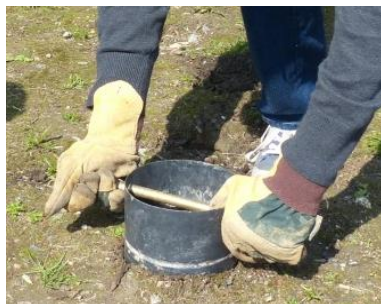
Figure 24: Carottage de sol
