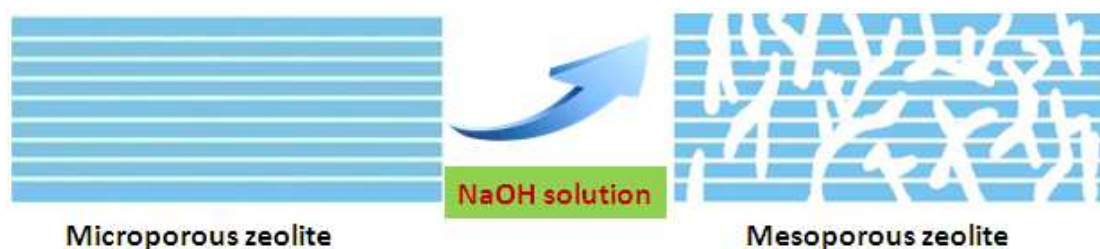
Figure 2-1. Diagram of introduction of mesopores into the microporous zeolite by desilication
