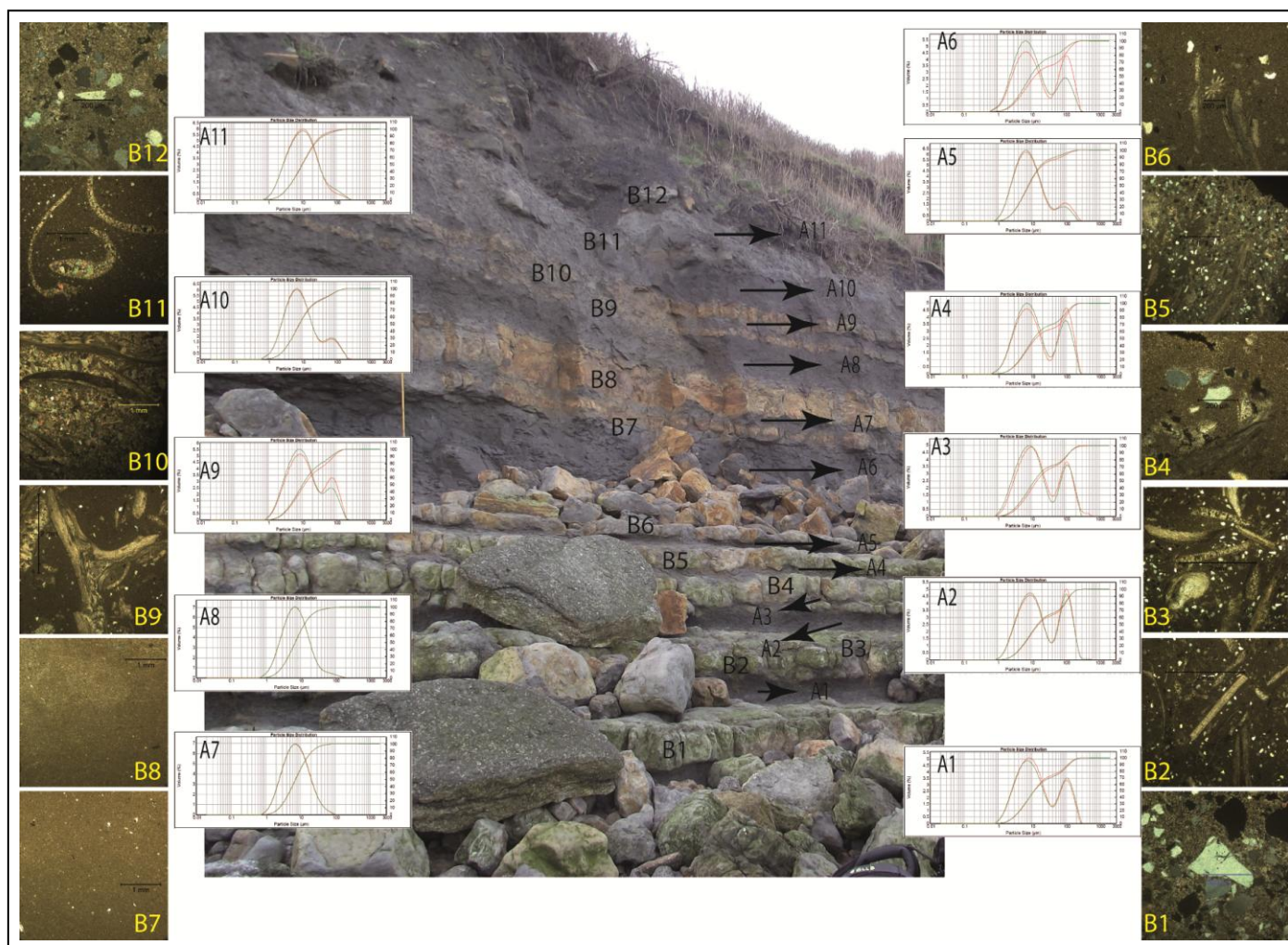
Fig. 9. Mosaic showing the grain-size distribution of the insoluble fraction of the marlstones (series A) and the microfacies of the limestone beds (series B) in the Calcaires du Moulin Wibert Fm. (Cap Gris-Nez).
