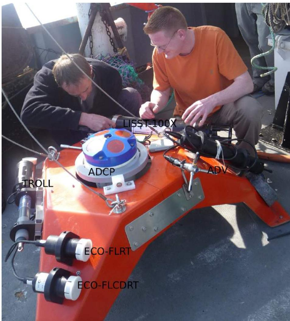
Figure 2.4: Instruments (bio-optical and hydro-graphic) mounted over the sea-spider for the in situ sampling; done in the laboratory of oceanology and geosciences, Wimereux.
