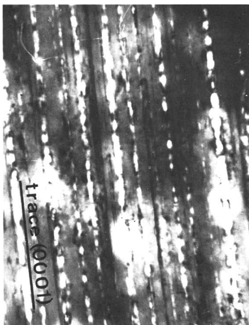
Figure 4.10: Magnesium irradiated at 3 \times 10^{21} \text{ n/cm}^2 ( E > 0.1 \text{ MeV} ). T = 55^\circ\text{C} . Foil normal: [11\bar{1}0] . Zoom \times 24000 . Voids are aligned as layers in the trace of the basal plane. The voids are randomly distributed in each layer (from [97]).
