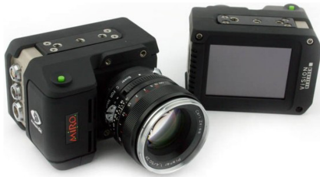
FIGURE 4.6: Phantom high speed camera is capable of capturing 1000 frames per seconds. The resolution of the camera is 512 \times 384 pixel and it is connected to a software called Phantom Camera Control application (PCC) (Benkeddad, 2015).
