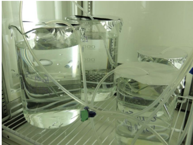
FIGURE 4.2: Culture of copepod species E. affinis in container conserved in incubator at temperature of 18 – 19°C with oxygenation and photoperiod 12h/12h. Salinity of water is 15 psu (Benkeddad, 2015).
