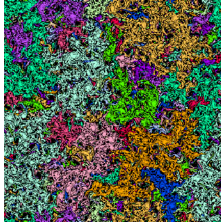
FIGURE 6.7: Colors identify different vorticity clusters and their boundaries are fractal with D_2 = 4/3 (Bernard et al., 2006).
