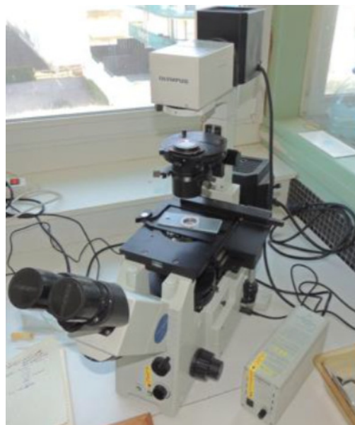
FIGURE 4.9: Olympus microscope connected to a software to calculate the size and identify the gender of copepod species (Benkeddad, 2015).
