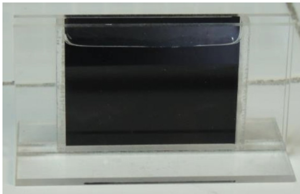
FIGURE 4.4: Experimental set up made of Acrylic with total volume of 8 ml and dimension of 63 \times 53 \times 6 \text{ mm}^3 in length, height and depth respectively (Benkeddad, 2015).
