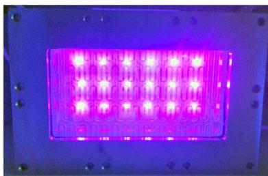
Figure 7.3: Lab designed HP UV LEDs A
