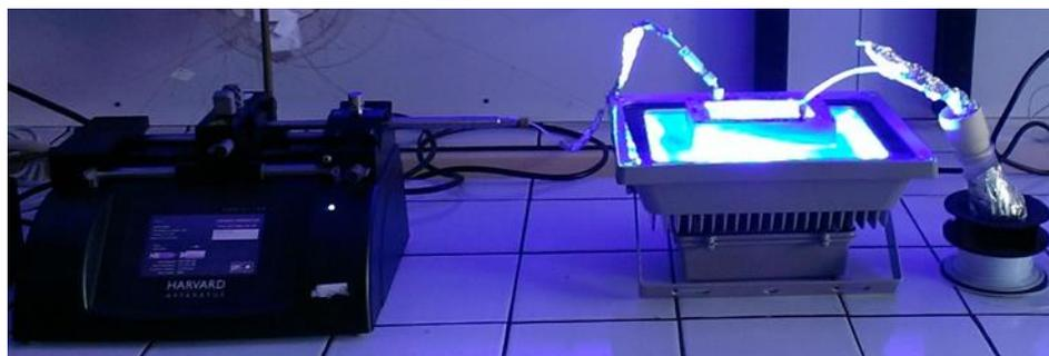
Figure 3.33: Set up for the photocycloaddition in flow using  $Ru(bpy)_3Cl_2$  and blue LEDs
