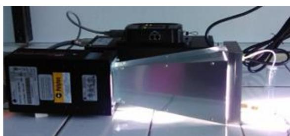
**Figure 2.10: Mikroglas Dwell device illuminated by HP LEDs B**
