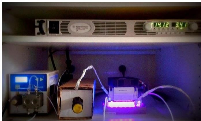
**Figure 2.9: Set-up of the photoisomerization of azobenzene under flow conditions using HP LEDs A**
