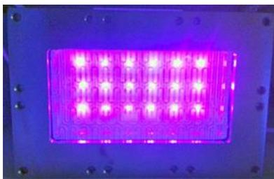
Figure 3.19: Mikroglas® Dwell Device illuminated by HP LEDs A 365 nm
