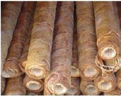
Figure 22: Cartridge Filter fouled by iron.
