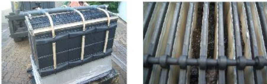
Figure 13: Sludge blocking between the plates due to faulty aeration system in the Flat sheet membrane.
