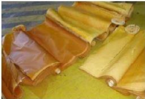
Figure 23: Membrane fouled by iron.
