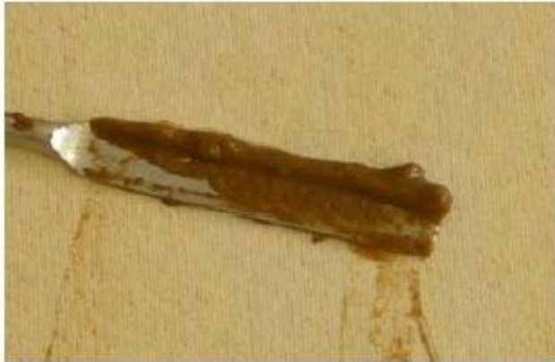
Figure 27: Membrane failure by Clay fouling [Chesters et al., 2011].
