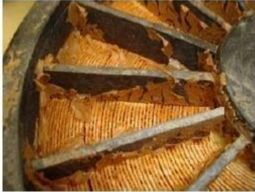
Figure 24: Membrane Fouling caused by iron acrylate [Chesters et al., 2011].
