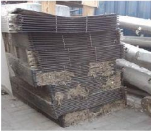
Figure 11: Damaged membrane to be replaced.
