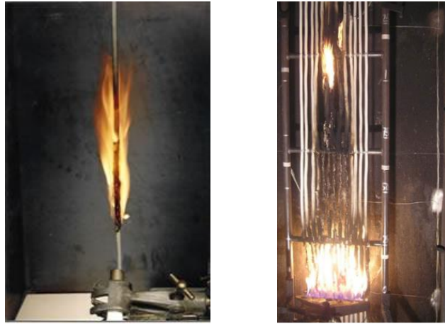
Figure 3: Cables tested in EN 50399 apparatus (right) and cable tested according to EN 60332-1-2 test (left)
