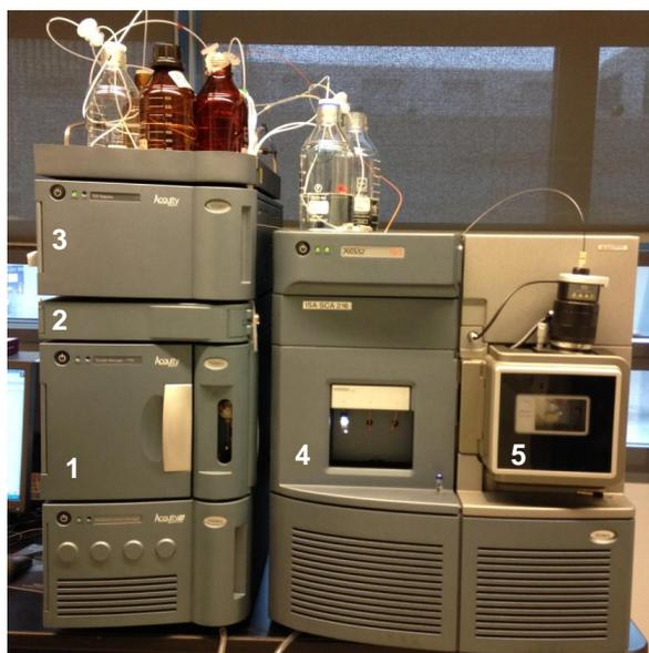
Figure S2.1: UPLC (Acquity H-Class) coupled with Xevo TQ-S (mass detector)
