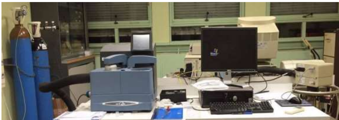
Figure 36. Equipment of DSC Q200.
