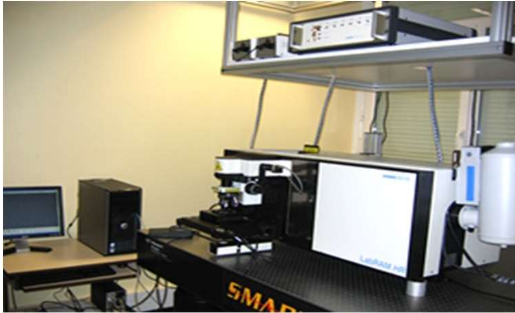
Figure 30. Image of the set up of a Horiba Yvon Labram HR Raman spectroscopy.
