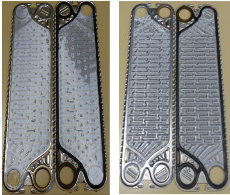
Figure 9. Pictures of the deposit layers on the surface of the PHE after conducting a 2 hours fouling experiment with either 0.25 (left) or 2.5% (w/w) (right) WPI model solutions.
