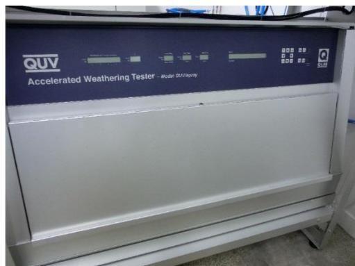
*Figure 31: Q-LAB, QUV/spray weathering chamber.*
