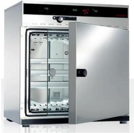
*Figure 30: Humidity chamber test HCP 108.*
