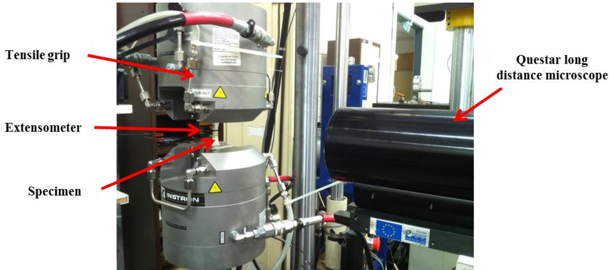
Figure 2-13: Experimental set-up with Questar microscope
