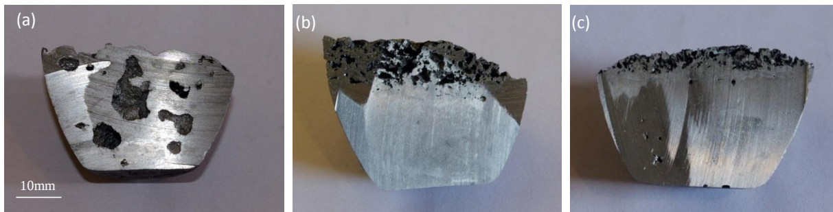
Figure 6-13: Porosity in the specimens at various degassing times with 1L/min argon (a) 0min; (b) 20min; (c) 35min
