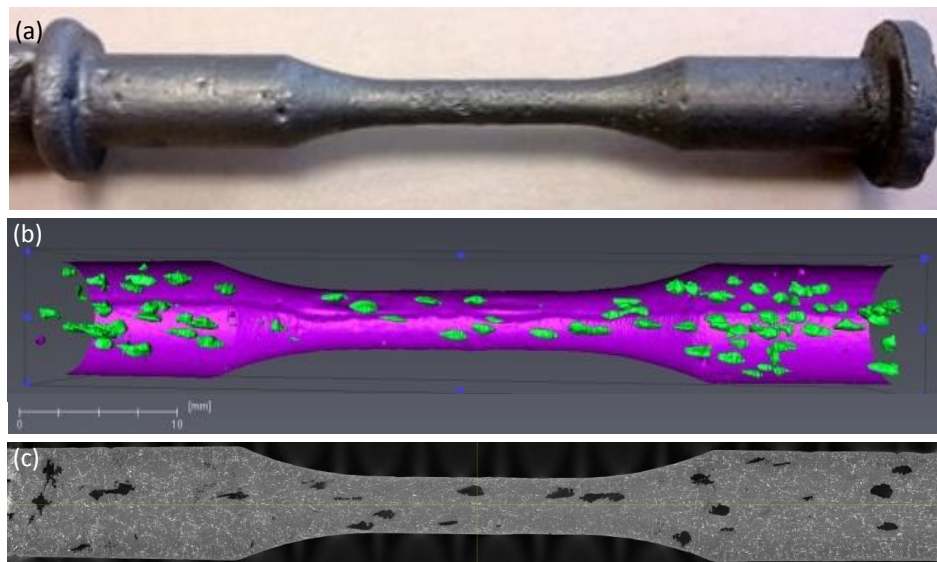
Figure 6-17: (a) Casting sample A, (b) 3D rendering of pores in sample A and (b) tomographic image slice showing the pore distribution
