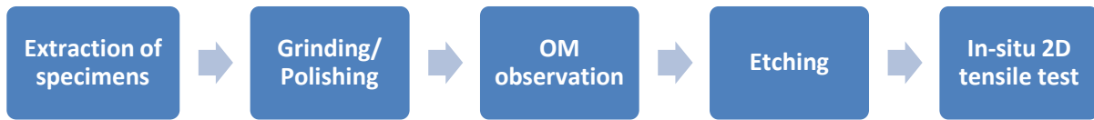
Figure 2-4: Scheme of specimen preparation for DC alloy
