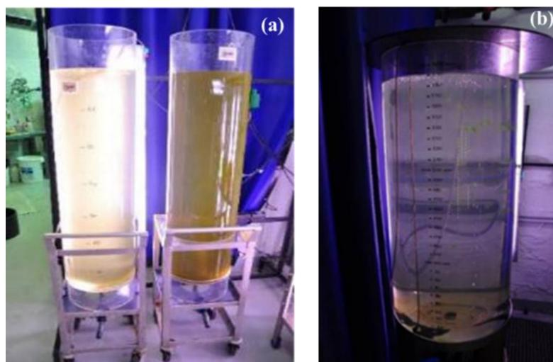
**Fig. 5.4** The mass culture system of copepods (a) 70-L for *A. royi* (b) 300-L for *A. tonsa*
