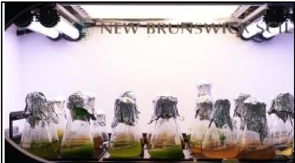
Fig.4.4. The regular cultivation method of Nostoc gelatinosum blue-green algae to undiluted wastewater from the exit of treatment plant in laboratory conditions.
