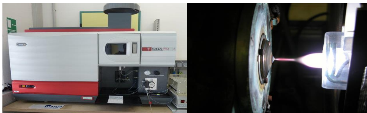
Fig. 2.8. Model ICP-AES (Varian Vista Pro) with its heating flame argon plasma at 6000K
