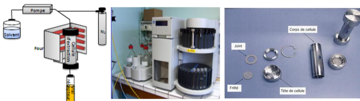
Fig.2.6. Simplified diagram of ESA, an actual photo and membership of an ASE cell
