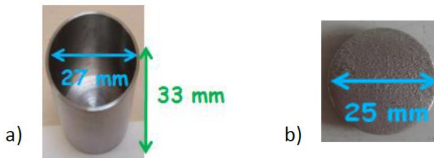
Figure 44. Sample holder (a) and top plate (b) used during rheological measurement
