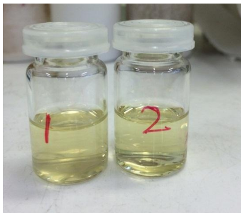
Figure 2-26 Pictures of the filtrates of reaction mixtures in epoxidation of cyclooctene catalyzed by \text{HPMo@MIL-100(Fe)} (Bottle 1 was from the first run, Bottle 2 was from the second run).
