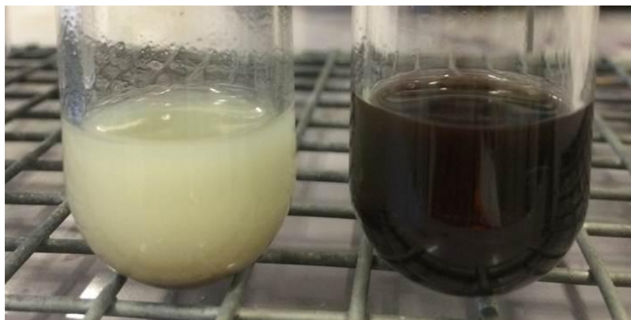
Figure 3-11 Pictures of the suspension of \{Mo_{132}\} with cyclooctene and ethanol at pH=10 (left) and pH=2 (right) before adding H_2O_2 .
