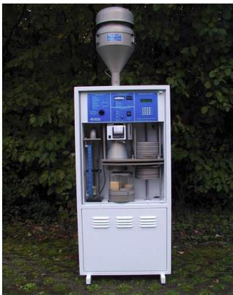
**Figure 23:** High-volume sampler Digitel DA80
