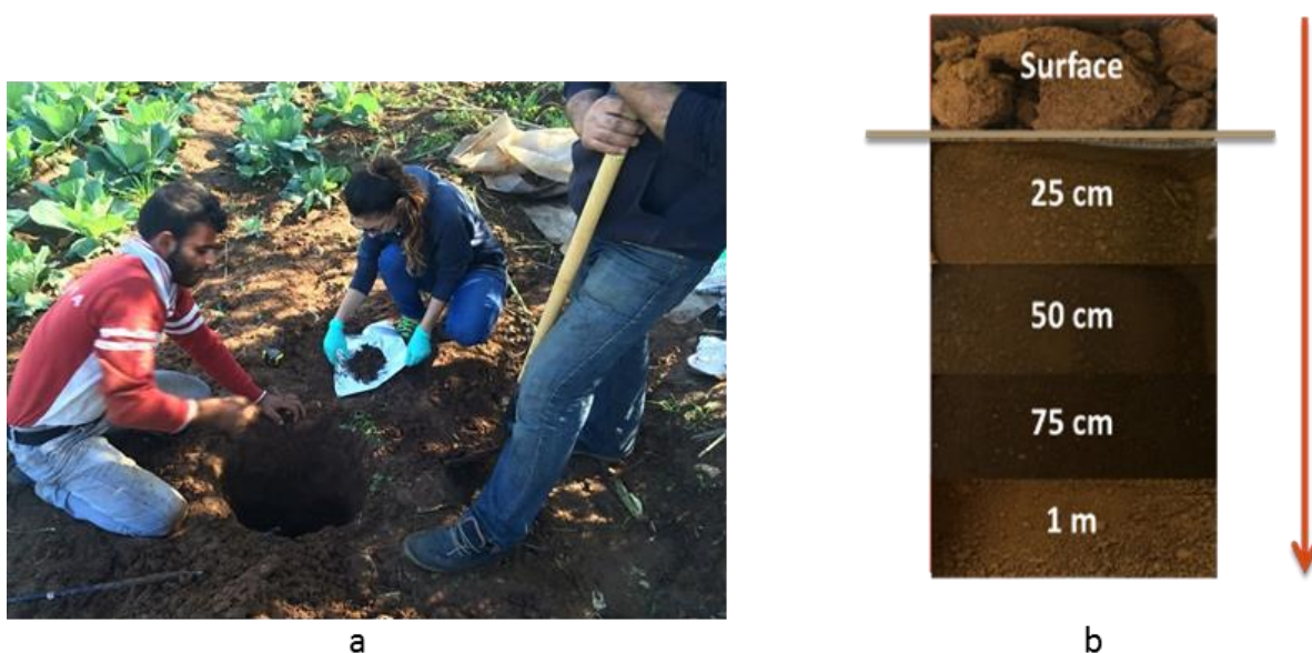
Figure 20 Soil sampling method (a) and different depth of studied area (b)
