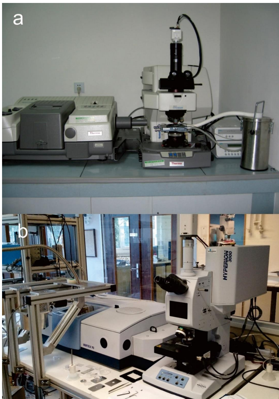
Figure 3-1. a) A photo of the Nicolet 5700 FTIR coupled with a Continuum microscope at CAS-CMME, USTC; b) The Bruker Vertex 70 spectrometer coupled with a Bruker Hyperion 3000 FTIR-microscope at University Lille 1, France.
